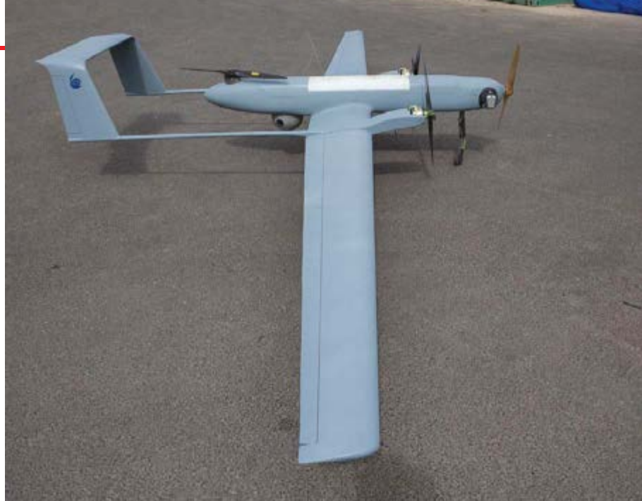
IAI's Panther family of UAS leverages tiltrotor technology to achieve vertical take-off and landing, then transitions the rotors for horizontal flight. (Photo: IAI)
